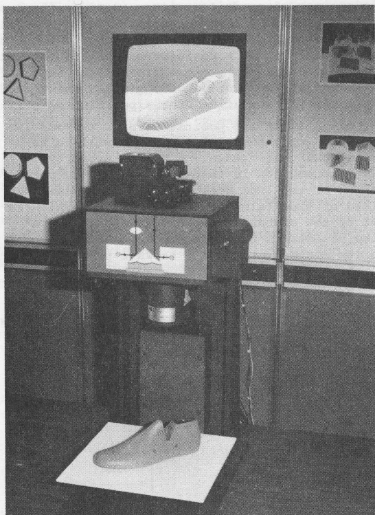
Figure 6. Photograph of the experimental prototype for high speed registered range-intensity imaging. The shoe last on the table is scanned in less than a second. More than 65,000 x, y, z coordinates are measured and displayed on a TV monitor.
