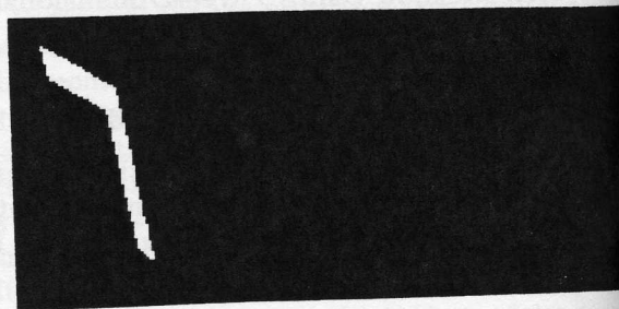
Figure 6: The planes extracted by region segmentation are shown here. Our approach then combines these planes with the edge information shown in Figure 5 to obtain the output shown in Figure 2.
