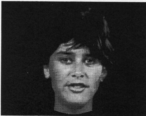
Figure 7: Frame 75 with the eyes and the mouth patches inserted from the codebooks. The right eye comes from frame 65, the left eye from frame 62 and the mouth patch is from frame 71.
