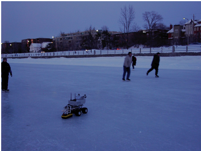
Image: robot measuring ice thickness with GPR on Ottawa canal (circa 2003)
