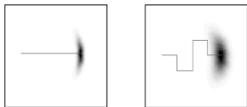
Fig. 1. The density p(x' | x, a) after moving 40 meter (left diagram) and 80 meter (right diagram). The darker a pose, the more likely it is.
