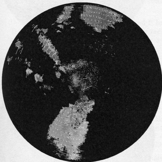
Figure 5: Computed full velocity flow field for real Doppler radial velocity dataset 200009251510 in a least squares framework using 7 \times 7 \times 7 neighbourhoods without smoothing.
