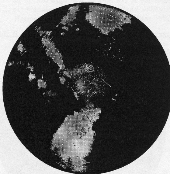
Figure 6: Computed full velocity flow field from real Doppler radial velocity dataset 200009251510 in a least squares framework using 7 \times 7 \times 7 neighbourhood with smoothing before the least squares computation stage.
