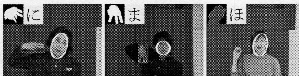
Figure 9. Example of the recognition of three different hand postures representing the phonemes “ni”, “ma” and “wo” respectively. In the rightmost image, the posture for “wo” was misclassified as the posture for “ho”, because the forearm of the subject is exposed and connected to her hand.
