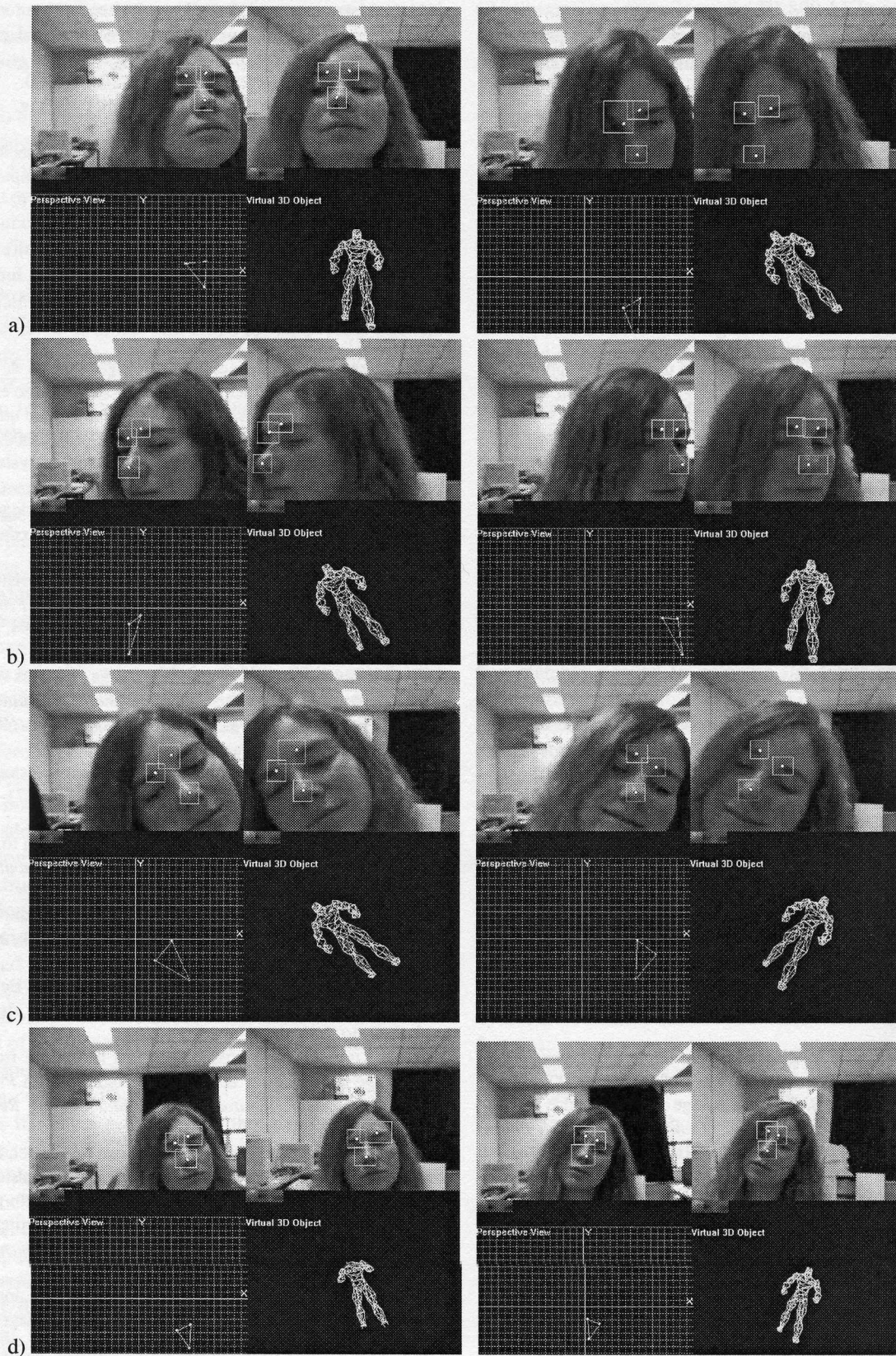
Figure 5: Snapshots of experiments showing the robustness and precision of the stereotracking accomplished with two webcams.
